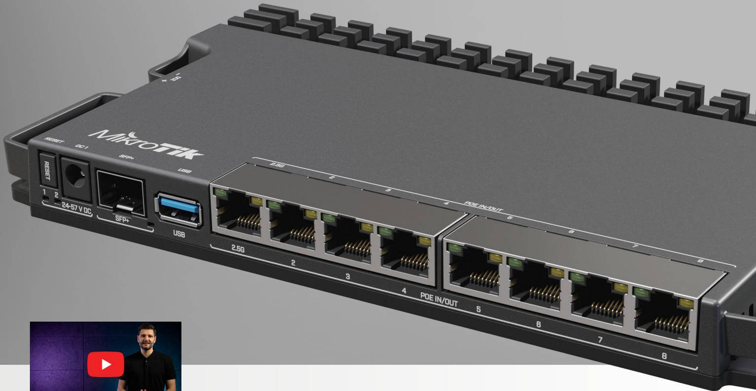
All power options support a **wide voltage range of 24 – 57 V**. However, you can not mix the voltages. If you're using PoE-out to power other devices, the board will choose the source with the highest voltage (DC jack or the 2-pin connector) to power those.
